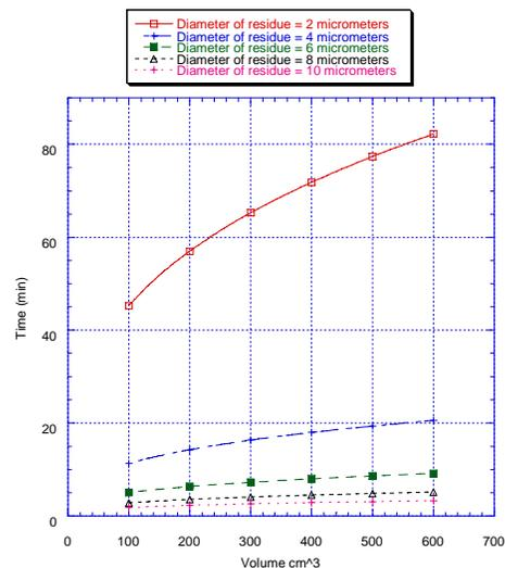
Figure 2: Sedimentation time for spherical Al<sub>2</sub>O<sub>3</sub> in ethanol at given volumes.
