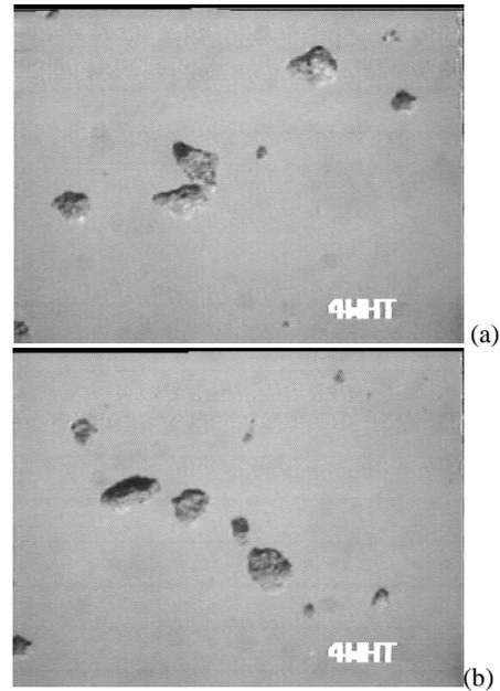
Figure 12: Images of ultra-fine Al particles at 5x1 magnification.
