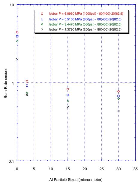
Figure 6: Burning rate versus Al particle size
