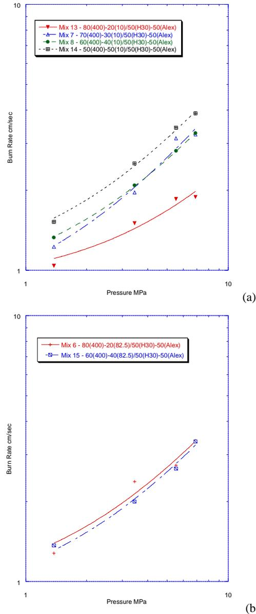
Figure 9: Burning rate vs. pressure for different AP c/f ratios for (a) AP = 10 $\mu$ m, (b) AP = 82.5 $\mu$ m.
