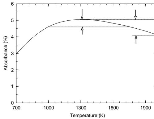
**Figure 4.** Temperature (in)sensitivity of the broadband absorbance for the conditions shown in Fig. 3 and a light source centered at  $4038 \text{ cm}^{-1}$ .
