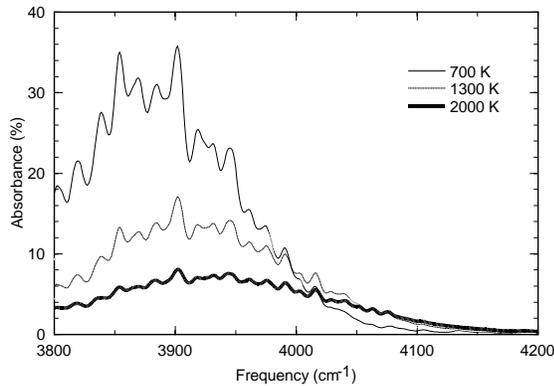
**Figure 3.** Overall absorbance for a broadband ( $10 \text{ cm}^{-1}$  Lorentzian) light source over a 5 cm path length in a uniform gas mixture at 10 atm, consisting of 5%  $\text{H}_2\text{O}$  by mole.
