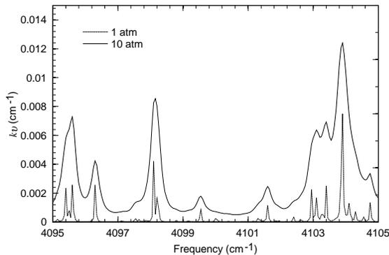
**Figure 1.** Spectral absorption coefficient  $k_v$  for a mixture containing 5% water by mole at 1300 K in a region above  $3800 \text{ cm}^{-1}$  for two pressures, 1 and 10 atm.
