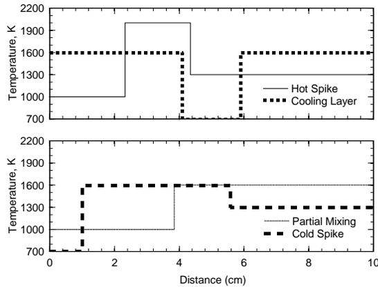
**Figure 7.** Profiles of temperature and water mole fraction across a 10 cm path through the exit plane of a combustor used to test sensor performance.
