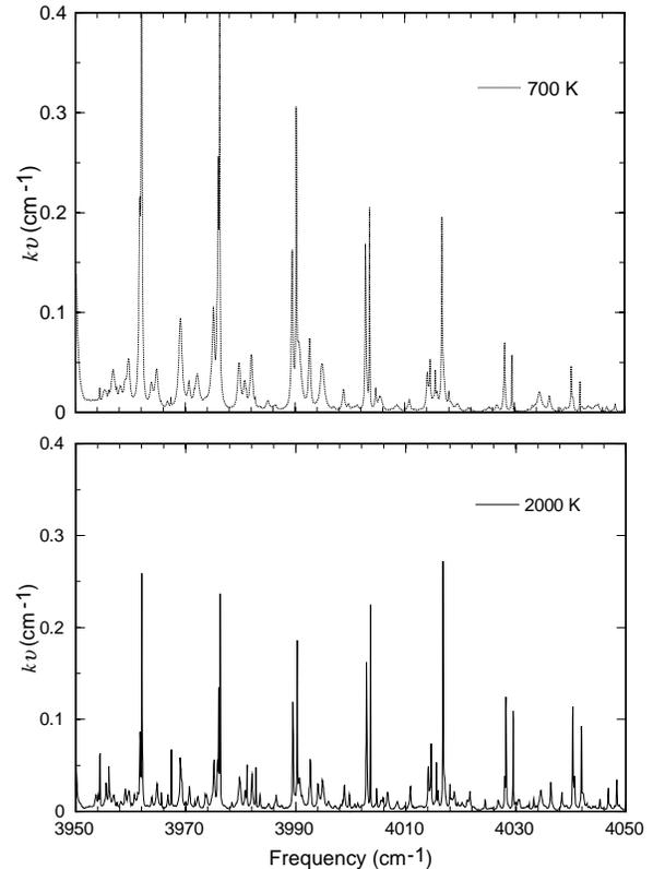
**Figure 2.** Spectral absorption coefficient  $k_v$  for 5% water at 700 K and 2000 K, and a pressure of 10 atm in a region near  $4000 \text{ cm}^{-1}$  that shows strong temperature dependence.
