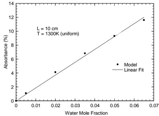
**Figure 5.** Variation in absorbance with water mole fraction for a  $10 \text{ cm}^{-1}$  bandwidth light source centered at  $4038 \text{ cm}^{-1}$  for uniform combustor exhaust conditions of 10 atm, 1300 K, and a 10 cm path length. The line is a best-fit to the calculated absorbances.
