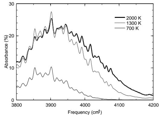
**Figure 6.** Overall absorbance for a broadband ( $10\text{ cm}^{-1}$  Lorentzian) light source over a 10 cm path length in a uniform gas mixture at 10 atm and various temperatures. The water content at each temperature varies linearly with temperature.
