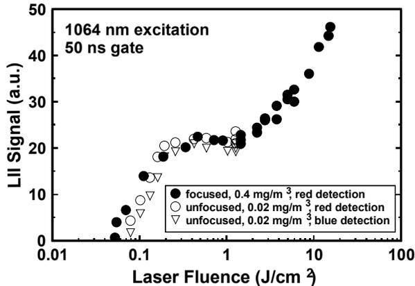
**Figure 9.** Prompt 50 ns integrated LII signals in the simulated exhaust versus incident laser fluence (IR). Signals are recorded with both the red and blue broad-band Schott glass combinations using  $0.02 \text{ mg/m}^3$  and an unfocused beam. Also plotted are signals acquired in the red using  $0.4 \text{ mg/m}^3$  and a focused beam.
