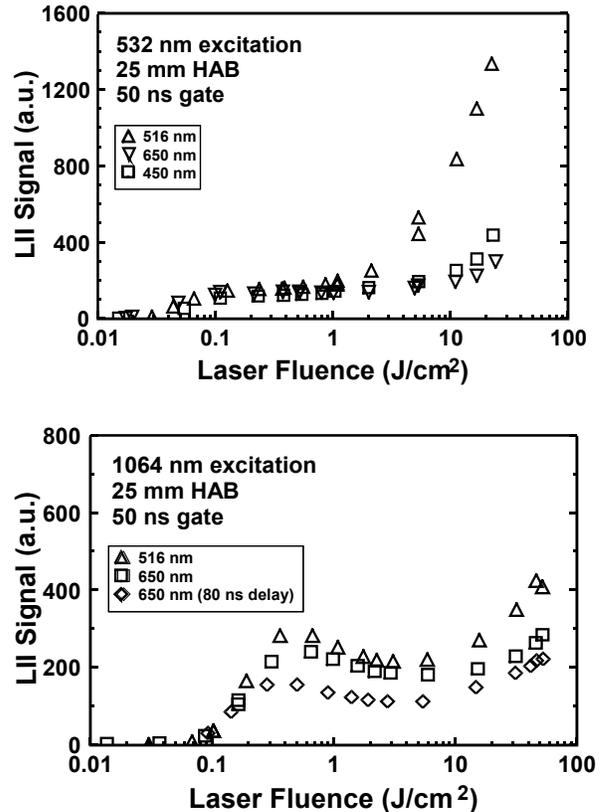
**Figure 8.** Prompt 50 ns integrated LII signals in the diffusion flame versus incident laser fluence. Signals are recorded at 650 nm, 430 nm and the  $\Delta v = 0$  Swan band head at 516 nm. Arbitrary vertical scales of the two plots are correct relative to one another.
