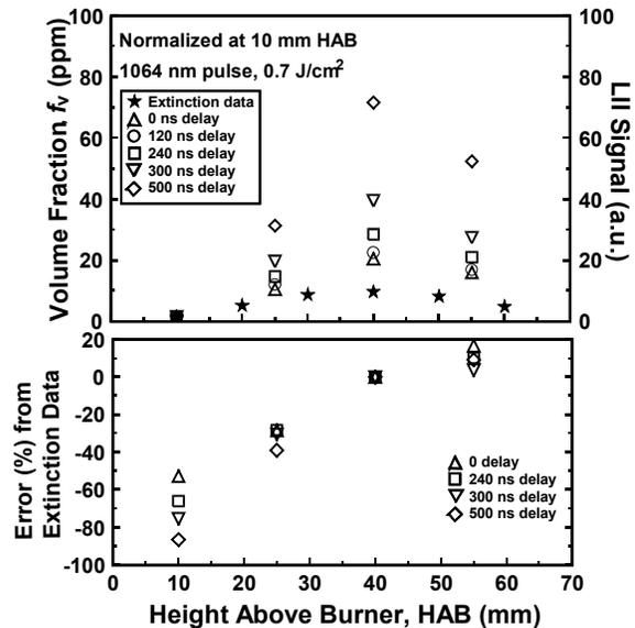
**Figure 4.** (above) LII signals generated at four heights in the diffusion flame, compared to extinction measurements of soot concentration.<sup>17</sup> Detection is at 430 nm. (below) Relative deviation of the LII signals from the extinction data. Renormalized at 40 mm HAB.
