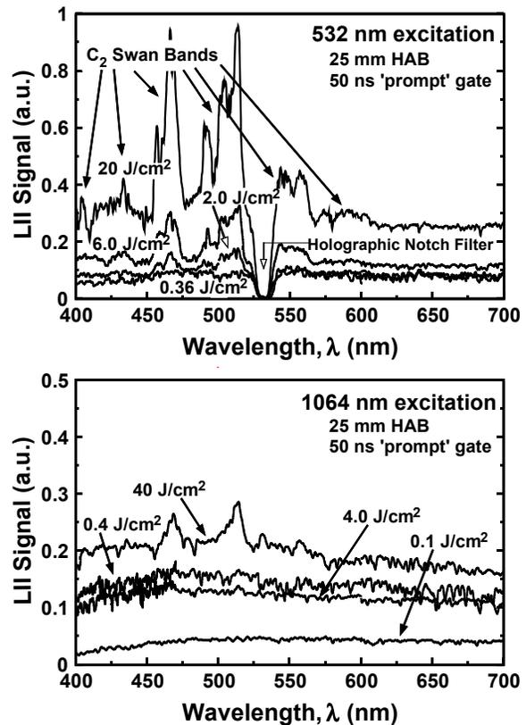
**Figure 7.** LII spectra recorded in the diffusion flame at a height of 25 mm. Visible wavelength spectra are shown for green and IR excitation and a wide range of excitation energies. The data are corrected for the response of the detection system and spectral emissivity of the soot particles.<sup>25</sup> Arbitrary vertical scales of the two plots are correct relative to one another.
