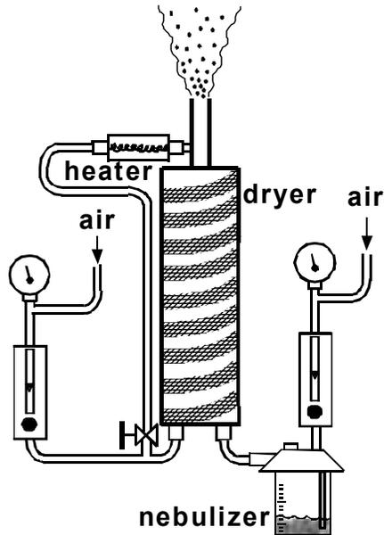
**Figure 2.** Soot generating experimental apparatus.. Dryer tube is wrapped with heater tape to maintain approximately 100 °C walls. Separate air flows are monitored with a rotameter and pressure gauge.
