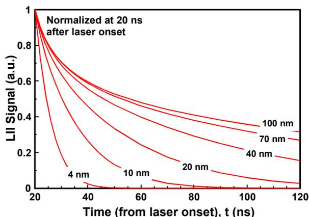
**Figure 1.** Model results for the signal decay from different sized particles illuminated by a  $0.5 \text{ J/cm}^2$  laser pulse at  $1064 \text{ nm}$ . Detection is at  $650 \text{ nm}$ . Ambient temperature is  $350 \text{ K}$ .
