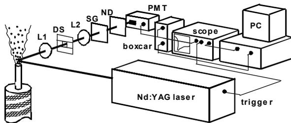
**Figure 3.** Laser-induced incandescence experimental setup (shown with soot generator). L1:  $f = 150$  mm lens, L2:  $f = 100$  mm lens, DS: height/width-adjustable rectangular aperture, SG: Schott glass filter(s), and ND: neutral density filter(s).
