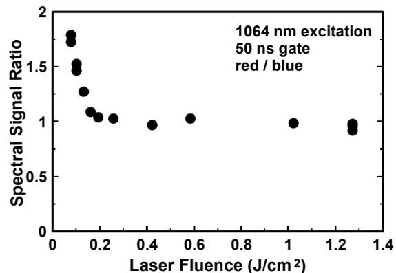
**Figure 11.** Ratio of red to blue signals recorded in Fig. 9 with the unfocused IR beam.
