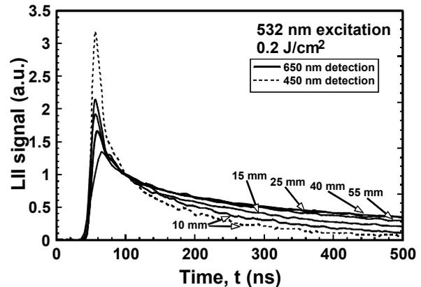
**Figure 5.** LII signal decay versus time for five heights in the ethylene flame and at two detection wavelengths. Primary particle diameters for these positions are 14, 22, 30, 33, and 31 from lowest to highest height.<sup>5</sup> Laser excitation is a Nd:YAG (532 nm) at  $0.2 \text{ J/cm}^2$ . Signals are normalized at 60 ns after signal onset.
