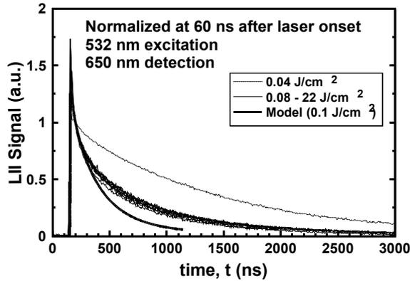
**Figure 6.** LII time traces for 40 mm HAB (33 nm particle) at various laser fluences. The broken line represents a case below the threshold intensity, while the solid curves range from threshold to over 200 times that fluence. The bold line represents a numerical simulation of the experiment at threshold ( $0.1 \text{ J/cm}^2$ ).
