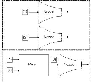
For this problem, assume both streams have the same molecular weight (28.85) and same specific heat ratio (1.39). Also assume that the amount of fuel burned produces a negligible change in the core mass flow rate, i.e., the mass flow rate exiting the core is essentially the same as that of the air that entered it, and that all nozzles are reversible, adiabatic and perfectly expanded.
