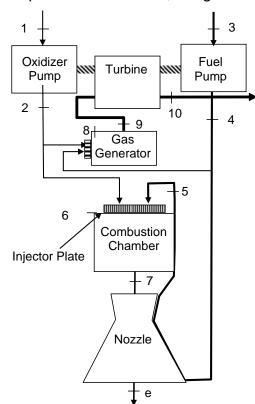
combustion chamber will be lower, just 14%. However, the fuel cooling loop will also require an additional 20% stagnation pressure drop ( $p_{04}$ =1.20× $p_{05}$ ). The liquid fuel injector for the gas generator will have a stagnation pressure sufficient such that its post-injection pressure matches the post-injection pressure of the oxidizer injector.
