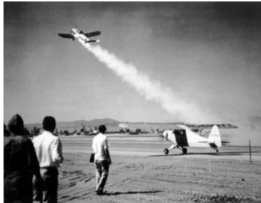
credit: National Air and Space Museum 1941 demonstration of Jet Assisted Takeoff (JATO)
